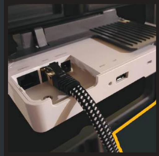
**9.** Connect one end of the ethernet cable to a port on the AP that takes the PoE input.
