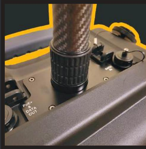
**8.** Connect the remaining poles. Unscrew the cap at the top of the case and screw in the lower pole assembly.
