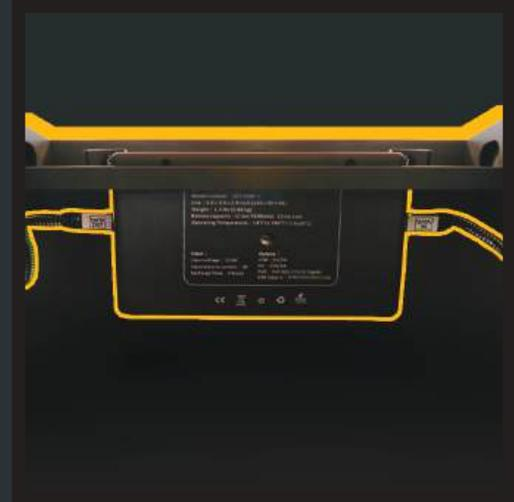
**3.** Plug in the PoE OUT cable to the PoE Output port on the left side of the battery, and if planning to connect the AP to data backhaul, plug in the DATA IN cable from the right side of the battery to its LAN port.
