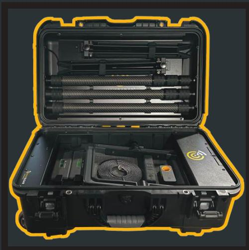
**4.** Remove the stabilizer legs, poles, mounng bracket, ethernet cable and any other tools you'll require for your survey.
