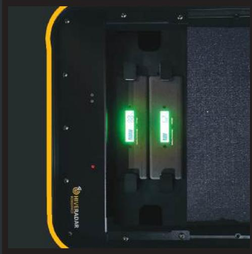
**2.** Insert the AccelTex Accelerator V2 batteries into the battery chasis in orientation so the battery specification text is facing the middle of the case, so the display is oriented also towards the middle.
